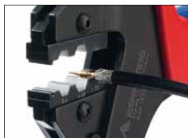
Innenleiter-Crimp Inner conductor crimp
