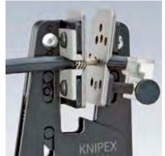
Automatic stripping of the insulation
