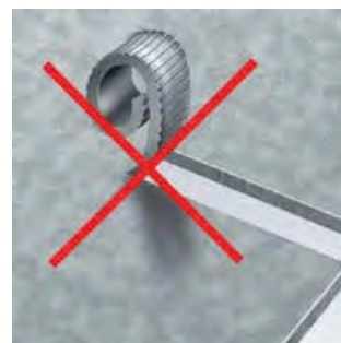
Notching without chip breaking
