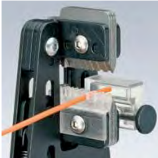
12 12 02 with cable guide and length stop
