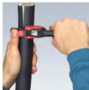
Turning the tool for circumferential cut
