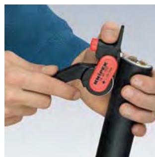
Setting the tool for longitudinal cut
